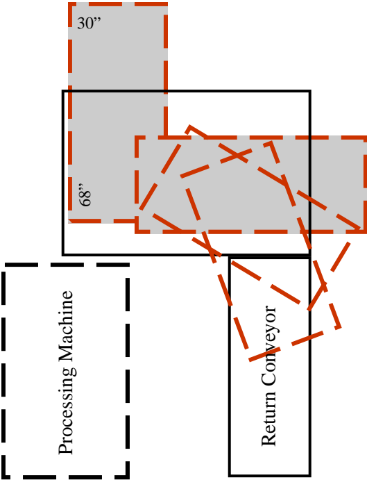
TB 48L x 72W w/24" Rollers Maximum part size is 30" x 68"
